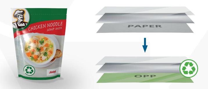
Paper can be substituted either with OPPalyte<sup>™</sup> white films (SHH) or Bicor<sup>™</sup> clear films with a matt-look (CSRM). Using non heat sealable matt OPP will help for packaging efficiency while providing a paper finish aspect.
